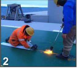
During cold, wet weather, it is highly recommended to heat the hatches using propane and a torch.
