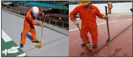
Sweep and make sure the hatch covers are clean, dry and dust free. In addition, use paint thinner with a rag to wipe off any loose grain, paint flakes, oil, salt or dust from hatch seams, then wipe dry.
